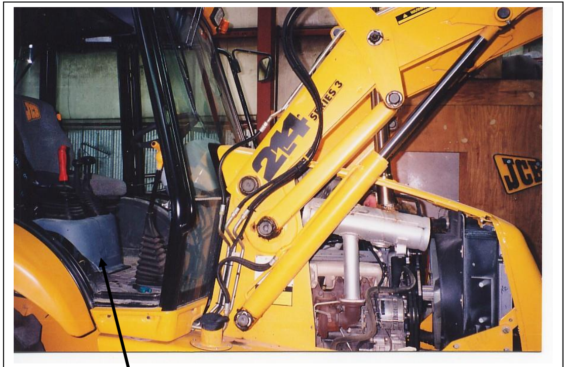
Plastic shroud over parking brake and loader control lifted up several inches
