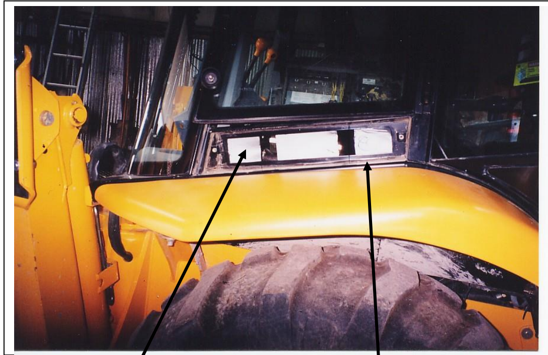
Foam Tape restricting outside air intake
